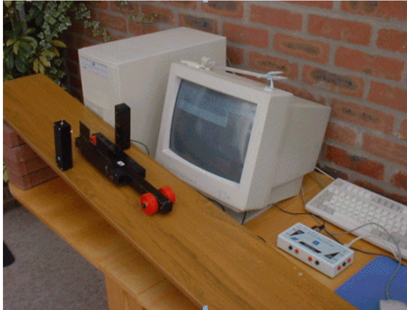
Figure 1 Investigating acceleration using a light gate
