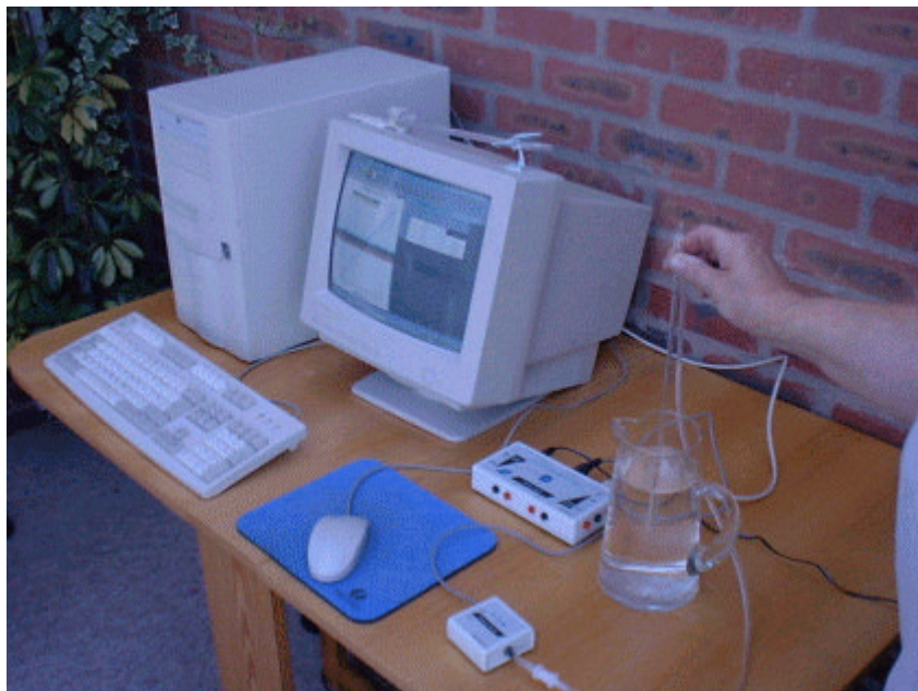
Figure 2 Investigating the variation of pressure with depth of immersion in water
