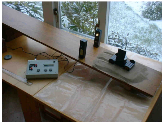
Figure 2 The TSA meter being used in an escape lane sand-trap investigation
